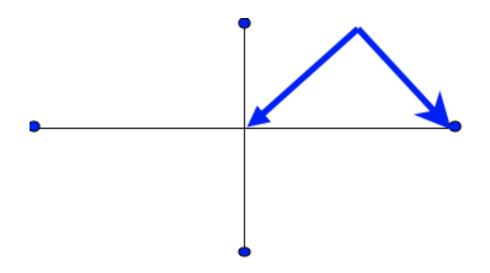
Next move the compass straight up the minor axis. Keep the point of the compass at the top of the minor axis and swing the pencil down and around (as in the diagram overleaf) and make a mark with the compass pencil as shown. Keeping the point in the same place, move it all the way around to mark the other side of the major axis as shown. These are the foci of the ellipse. For a planet orbiting a star, the star would be at one of these foci.
