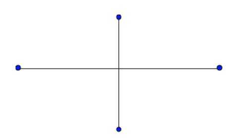
To start drawing the ellipse, stretch the compass from where the axes intersect to the end of the major axis.
