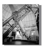
The telescope is a refractor which means it has a glass lens that bends light to form an image – this lens is 28 inches wide (71 cm) and can achieve magnifications up to 300 times. The telescope has an equatorial mount whereby the telescope is tilted at an angle equal to the latitude of Greenwich. It is driven by a motor that matches the Earth's rotation allowing the telescope to track objects as they appear to move. The telescope is now used for public evening sessions.
